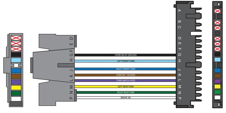
Plug this end into the steering column
